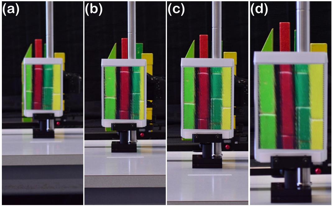
FIG. 4. (a)-(d) **Integral cloak longitudinal ( $z$ ) demonstration.** Observer (camera) at different distances in front of the display screen of the cloak: 272 cm, 235 cm, 203 cm, and 150 cm, for (a)-(d), respectively. As expected, the cloak displays more of the background objects, spatially, for closer observation.
