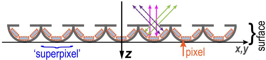
**FIG. 5. Lensless ‘integral cloaking’ surface.** Cross-section view shown. Detector and/or display pixels can be placed on curved ‘superpixels.’ The top layer, which has holes for rays to pass, can be made to absorb light, or also detect incident light to calculate and compensate for irradiance losses.
